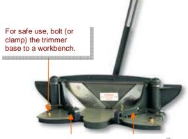
Fences set at 45°. The back of the moulding should run against the fence.
