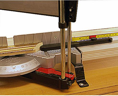
The nose of the stop reaches in over the saw-table which allows framing of very small pictures.
